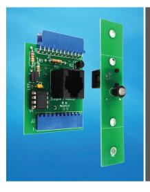
The StarGate-III Indicator device provides a mechanical interface to the RADC. This direct connection enables zone status information to be displayed remotely via a wall-mounted LED component.
