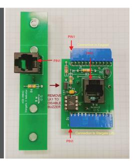
The remote LED board is easily connected to the main Indicator module using a 4 conductor 1-to-1 RJ11 cable
