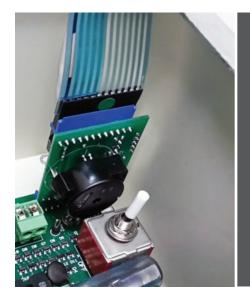
The side of the main Indicator module containing the alarm Buzzer must be positioned toward the StarGate-III power switch
